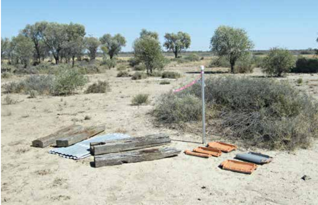
Figure 2.1 Example of artificial substrates—corrugated iron, railway sleepers and roofing tiles—used to sample herpetofauna at a plot within a site
