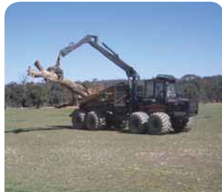
Figure 17.3: A forestry forwarder drops logs into Goorooyarroo Nature Reserve. Photo: A. Manning
