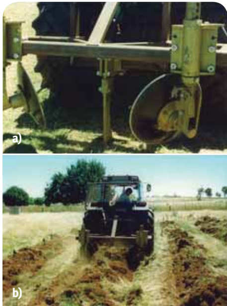
Figure 15.6: a) A tractor-mounted ripper-moulder showing ripping arm and mounding discs. b) Ripped and mounded soil after one pass. Some applications will require two passes. Photos: D. Carr
