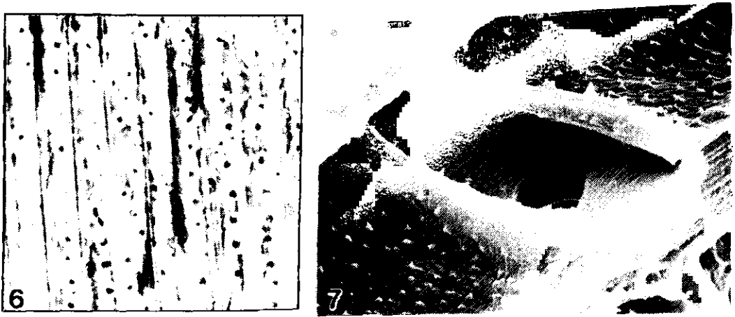
Figure 6. Photograph adapted from page 178 of Baker and Smith (1910) and which has the caption: 'Radial section through the timber showing the bordered pits of the tracheids. Callitris intratropica \times 120 '.
