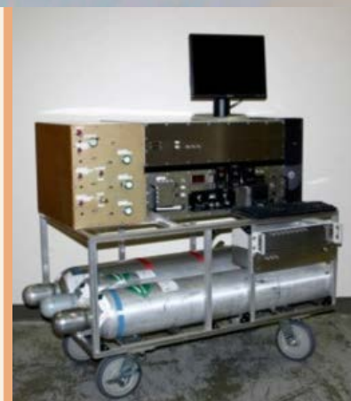
Click to enlarge image. The Carbon Isotope Laser Absorption Spectrometer (CILAS) will provide in situ measurement capability to study 'fast' carbon exchange processes involving 13 C/ 12 C CO 2 isotopes, and may be operated in the field continuously for long time periods (hours to days).
