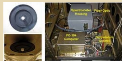
Figure 2. Zenith and nadir optics and instrument rack on the NASA DC-8 aircraft during ARCTAS.
