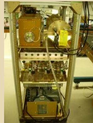
Figure 1. The CARI Fast-O 3 and CO instrument combined in one aircraft rack, ready to be installed on the NCAR/NSF GV aircraft in support of the START-08 mission.
