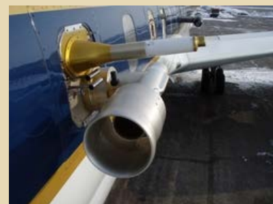
Figure 2. Inlet configuration for HO x instrumentation on the NASA DC-8 during ARCTAS (2008). The top inlet is for peroxy radicals, and the bottom one is for OH and sulfuric acid. The small stainless tubes provide air inlets that are used to generate ions that are exposed to the sampled air.
