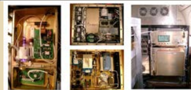
Figure 2: The NCAR Airborne Oxygen Instrument (AO2) measures O 2 concentration (reported as O 2 :N 2 ratio) using a vacuum-ultraviolet absorption technique. It consists of a pump module, a cylinder module, and an instrument module - High resolution figure
