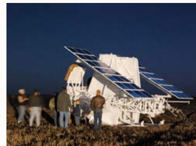
The Sunrise gondola being retrieved after landing in a flat, newly harvested wheat field. The gondola sustained a little damage to the roll cage but the telescope remained unharmed.
