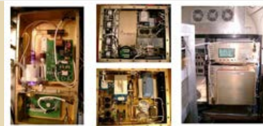
Figure 2: The NCAR Airborne Oxygen Instrument (AO2) measures O 2 concentration (reported as O 2 :N 2 ratio) using a vacuum-ultraviolet absorption technique. It consists of a pump module, a cylinder module, and an instrument module.
