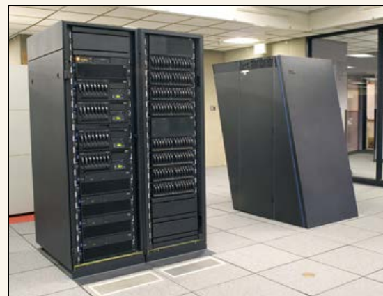
The IBM Blue Gene/L computer at NCAR (right) is designed for high performance and low power consumption. CISL and its collaborators performed significant R&D to make it a useful tool for geosciences research. Frost is now operating at a high level in multiple roles for universities, NCAR, and the TeraGrid.
