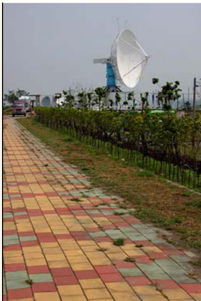
S-Pol, EOL's transportable, ground-based Doppler radar, on site for Terrain-influenced Monsoon Rainfall Experiment (TIMREX) in Taiwan.
