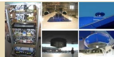
Figure 3. HARP rack installed on the NSF HIAPER GV aircraft, irradiance and actinic flux zenith and nadir optics.
