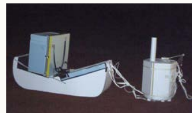
The Driftsonde "sled" carries the gondola (left) and the balloon control system (right.)
