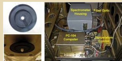
Figure 1. Zenith and nadir optics and instrument rack on the NASA DC-8 aircraft during ARCTAS.
