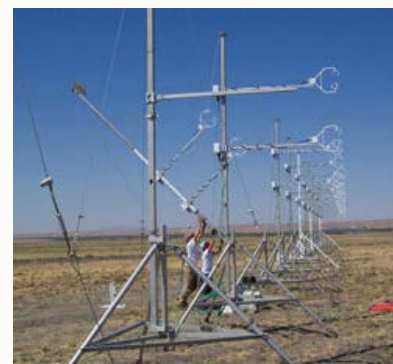
Setting up for AHATS: An array of sonic anemometers perched on tripods collected data on atmospheric turbulence close to the earth's surface.
