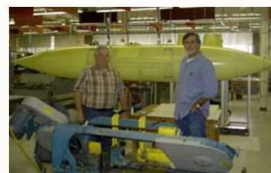
DFS staff stand in front of a complete GV Wing Pod. Notice the windows, that were being cut in the photo above, in the central portion of the pod.
