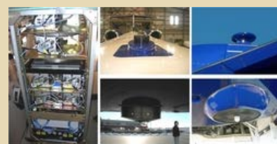
Figure 1. HARP rack installed on the NSF HIAPER GV aircraft, irradiance and actinic flux zenith and nadir optics.
