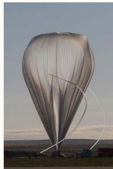
Slender hoses, blown into arcs by the wind, partially fill the balloon with helium before the Sunrise Solar Telescope launch. A large portion of the balloon is left unfilled so it can expand as it ascends into the stratosphere, where air pressure is considerably lower.
