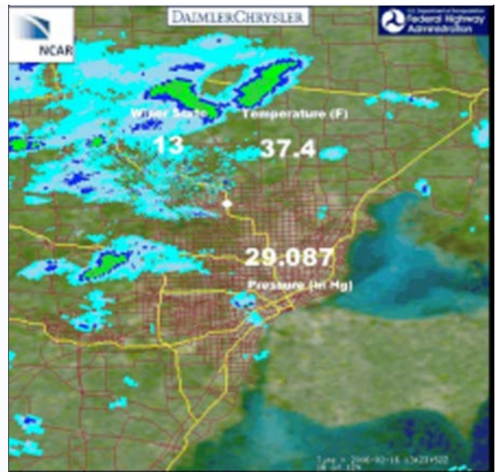
Example of a passenger vehicle traveling in Detroit wirelessly exporting weather measurements during a day with thunderstorms. Data courtesy of Daimler Chrysler
