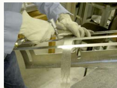
A machinist in the DFS Machine Shop hand-cuts windows in the GV Wing Pods. A full sheet of metal must be cut and shaped before the windows are cut, otherwise the integrity of the metal would be destroyed.
