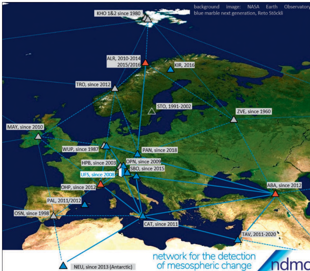
Fig. 8: European part of the NDMC network. Blue triangles denote stations, which are equipped with a standard GRIPS and/or FAIM instrument (as shown in Fig. 4 (b), (e), (f) for the UFS); red triangles show stations which in addition to a GRIPS or FAIM also host other independent instrumentation aimed at observations in the mesosphere; grey triangles denote stations with different airglow instrumentation; stations with temporary observations are marked by open triangles (background image credit: NASA Earth Observatory, excerpt from blue marble next generation (August), Reto Stöckli).
