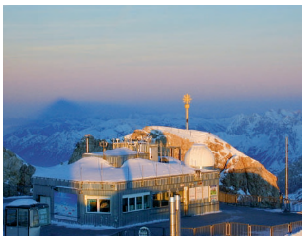
Fig. 1.1: The solar FTIR observatory at the Zugspitze summit (2964 m.a.s.l.) as a contribution to the international networks NDACC and TCCON. The optics dome opens during clear sky conditions and a computer controlled solar tracker redirects the solar beam into the FTIR spectrometer inside the building.
