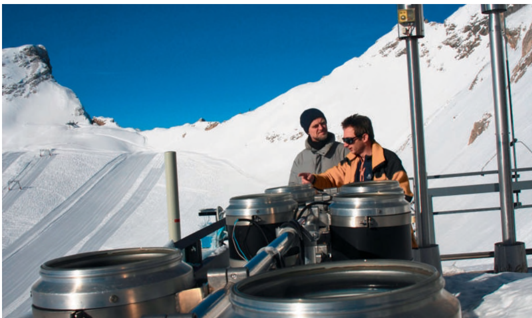
Fig. 6: Heated funnel adsorber deposition samplers which are used at the UFS. Picture: KF, LfU
