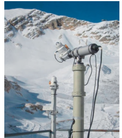
Fig. 5: Measurement of the UVI on tilted surfaces in the skiing area at Zugspitze-glacier with the system ASCARATIS, described in the text. Shown are the moving radiometer, which needs some time to observe all directions, and the radiometer that is permanently in horizontal position to check for unchanged illumination during the observation time. (Oppenrieder et al., 2004)
