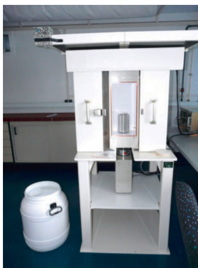
Fig. 6: HPGe broad energy gamma spectrometer system (left) at the Environmental Research Station Schneefernerhaus (Photo: K. Hürkamp, 2011-10-19). Detector cooling is performed with an electronically powered cryostat. An active veto shield (plastic scintillators) on top of the lead shielding provides additional reduction of the background due to elimination of altitude-induced enhanced cosmic radiation by a factor of 1.9 to 2.2. The right figure shows the measured background spectra with and without active veto-shield.
