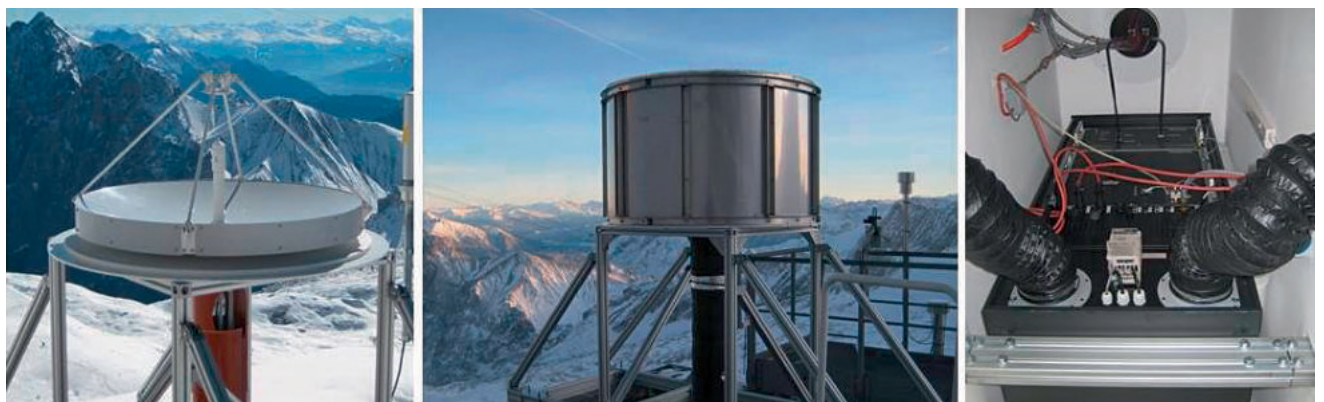
Fig. 2: Installation of the MIRA36 cloud radar at Umweltforschungsstation Schneefernerhaus. Left: antenna of Cassegrain type during the installation phase with parabolic dish, feed horn in the center and sub-reflector at the top. Center: antenna with clutter fence. Right: radar transmitter and receiver within the suspended ceiling of Wechselnutzlabor. Photos by M. Hagen.
