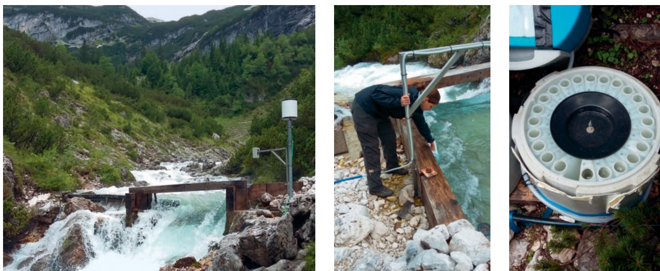
Fig. 4: Partnach gauge 200 m downstream the Partnach spring. The station is equipped with sensors for the determination of surface water discharge parameters (left) and an automatic water sampler (right). In addition grab surface water samples were taken (middle) during the summers 2015 and 2016 (Photos: K. Hürkamp, 2016-07-12).
