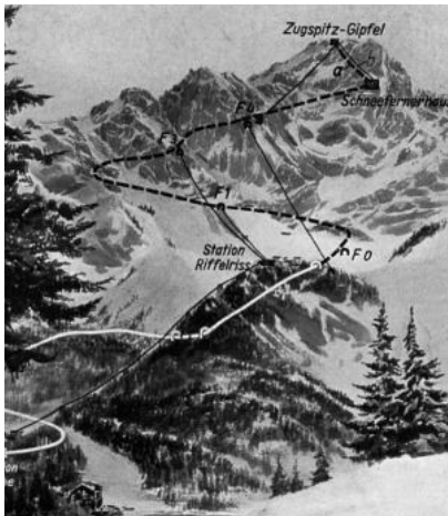
Fig. 10: Tunnel course of the planned cogwheel railway in the interior of the Zugspitze
