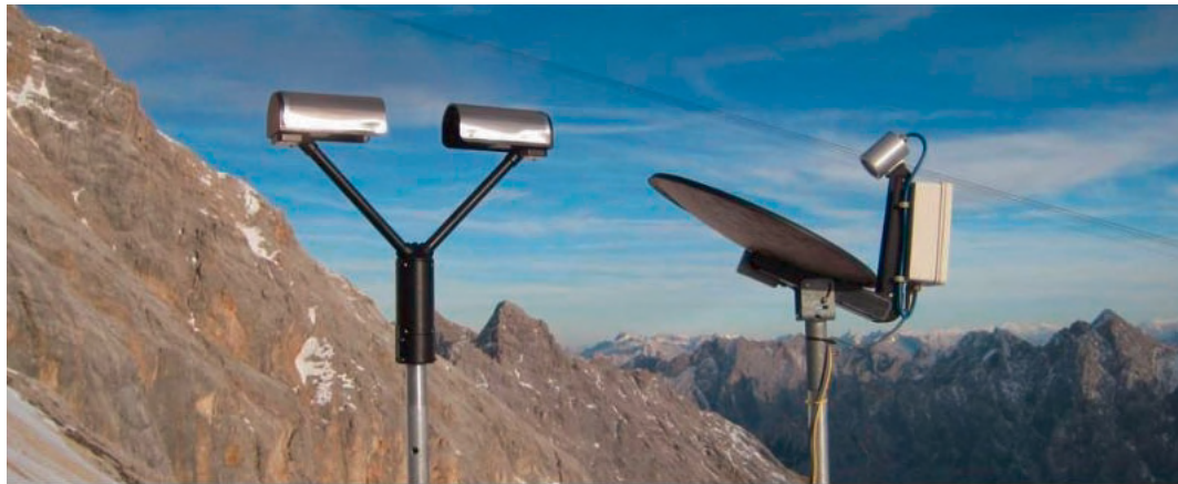
Fig. 3: Installation of the PARSIVEL-2 disdrometer (left) and MRR micro rain radar (right) at the top terrace of the Umweltforschungsstation Schneefernerhaus. Photo by M. Hagen.
