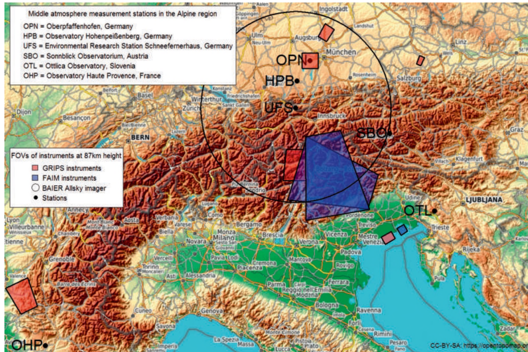
Fig. 9: Alpine observatories which are equipped with airglow instrumentation and their respective fields of view in the Mesopause region (state: 2018). The red areas show locations of spectrometric observations, the blue areas show areas observed with imagers, the large circle denotes the area, which is effectively observed by the BAIER all-sky imager from the UFS. FAIM 1 (OTL) and FAIM 4 (OPN) target the same area, thus allowing the study of dynamical features under different viewing geometries, so-called stereoscopic imaging (map credit: https://opentopomap.org , license CC-BY-SA).
