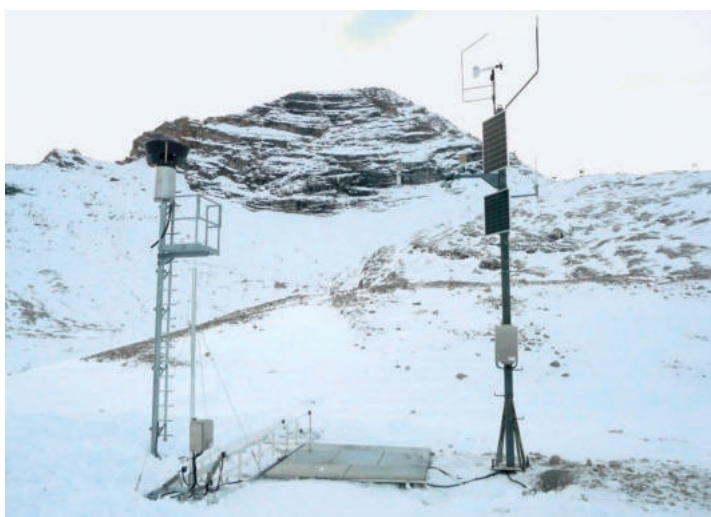
Fig. 8: Meteorological station at central Zugspitzplatt (2420 m a.s.l.), operated by the Bavarian Avalanche Warning Service and the authors on behalf of the Environmental Research Station Schneefernerhaus. It is equipped with sensors for the determination of standard meteorological and snow parameters. The measurement data is recorded and transferred to the Alpine Environmental Data Analysis Center (AlpEnDAC, www.alpendac.eu ), where it is publicly available (Photo: F. Bernauer, 2012-11-08).
