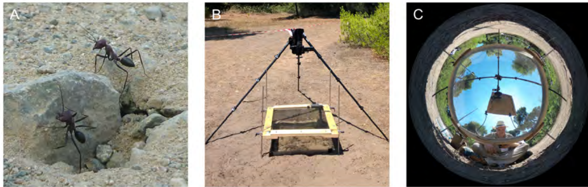
FIGURE 1 | Experimental setup for skylight manipulation experiments. (A) Unmarked C. noda ants at the nest entrance. (B) 30 cm above the nest entrance, a filter was placed in order to alter the skylight information. Learning walks were recorded with a high-speed 4K-camera. In addition, a HD-camcorder recorded the nest entrance for the whole day. (C) Panoramic image of the UV-block with sunshade setup (UVBS). The observer was located in the south to trigger the high-speed recording and to prevent unmarked ants from leaving the area covered by the filter through the opening in the fence, which was located in the south-west.
