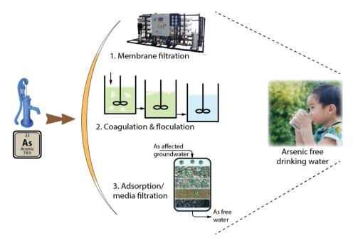
Fig. 4. Common technologies suitable for small-scale treatment of arsenic contaminated groundwater for potable water provision.
