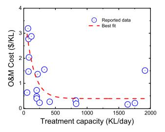
**Fig. 5.** Relationship between the unit cost of operation & maintenance and treatment capacity of adsorptive media filtration systems for arsenic removal in the US.
