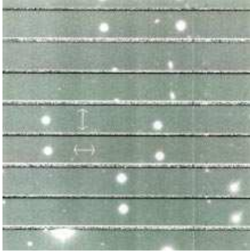
Figure 1: Example of a CCD frame obtained with EFOSC2, a Wollaston prism in the grism wheel and a mask at the focal plane of the telescope. Every object in the field has two orthogonally polarised images separated by \sim 20'' and called upper and lower images in the text. The arrows illustrate the direction of the polarisation of the two images. The y-axis is defined along the columns of the CCD, which is roughly the direction of the splitting. The detector was the Loral/Lesser CCD #40 with a pixel size of 0.160'' on the sky. The target was the quasar M08.02, observed on April 27, 1998 in the V filter with an exposure time of 300 s. It has a degree of polarisation p \simeq 1.4\% .
