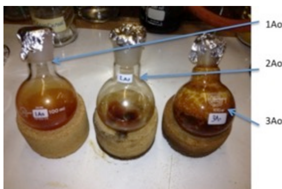
Figure 3-11 A digital image of Agelas oroides extracts in round bottom flasks. (hexane extract (1Ao), acetone extract (2Ao), methanol extract (3Ao))
