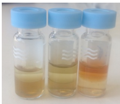
Figure 5-6 Digital image of marine sponge extracts suspended in biphasic systems along HEMWat scale. A visual difference was readily observed in the phase location of antibacterial products, which was confirmed by TLC.
