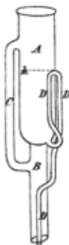
Figure 3-8 Soxhlet's original drawing of his extractor. (A) Central reservoir containing paper thimble and dry sample, condenser positioned above, causing volatilised solvent to slowly drip into sample; (B) Solvent positioned in heated beaker below; (C) Solvent evaporates and rises through column before condensing into central reservoir; (D) Syphon allowing recirculation of solvent (W. B. Jensen 2007).
