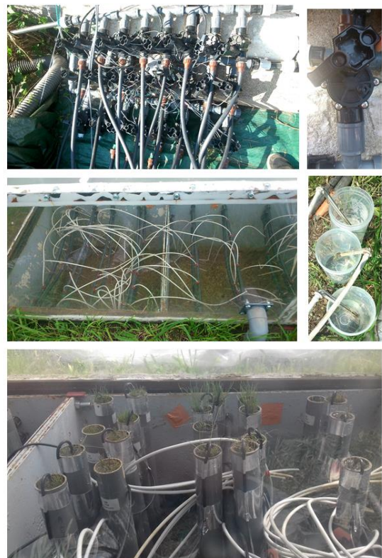
Figure V1-P2.2: From top to bottom row: Individual valves, water outlets in the greenhouse and irrigation pins to measure water amounts, final set-up with pots
