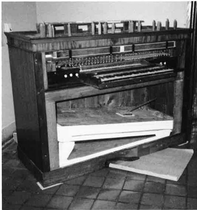
Restored, the organ was photographed before the top of the case was erected. The restored bellows and feeder, dating from ca. 1765, resides in the bottom of the case where it is pumped via the pedal emerging from the front.
