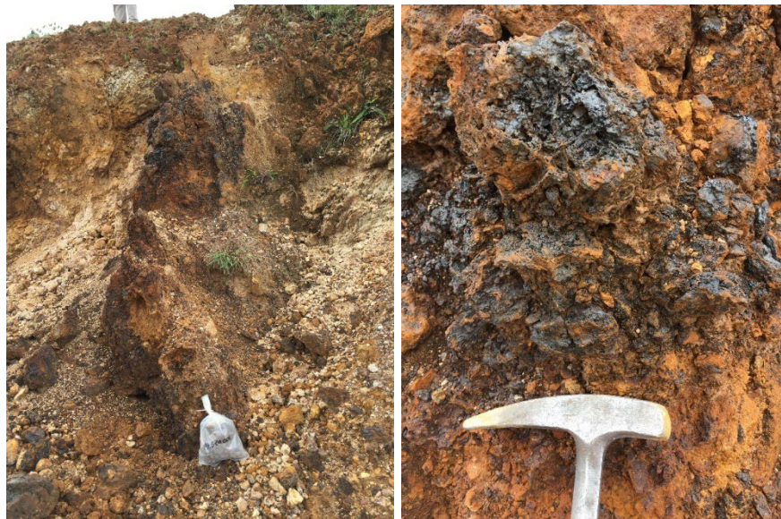
Figure 7-12 Iron oxide stained, locally gossanous vuggy silica exposed in surface cut, Quema-Quemita zone. Left: outcrop. Right: detail of gossanous breccia. (M. Gray, 2017)
