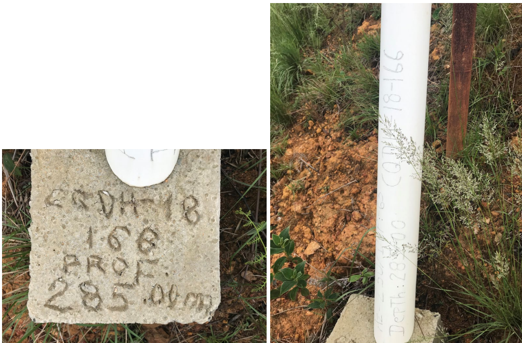
Figure 12-5 Example of Drillhole Collar Location (MMTS, 2021)
