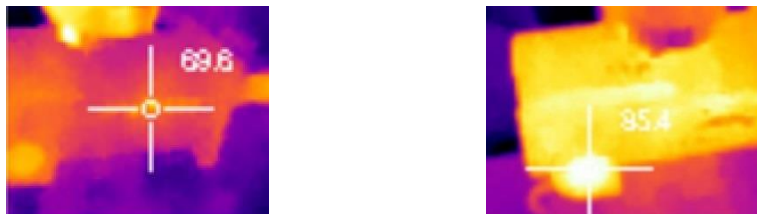
Figure 5: Infrared camera image for a motor – the crosshair identifies the location for estimating the surface temperature – Motor at 69.6 °F (left image) and at 85.4 °F (right image)
