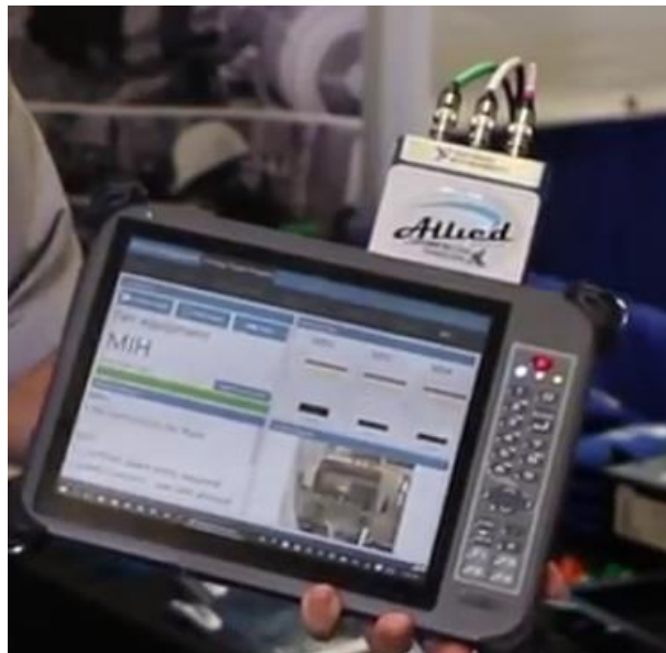
Figure 12: AR-C10 device with three sensors connected to it.
