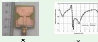
Fig.3. Photograph of the band notched staircase shaped UWB antenna (a) Photograph. (b) Measured and simulated return loss.
