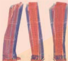
Fig. 3. First three modes of the Al-Hamra Tower model(6.5, 4.8, 2.9 sec)
