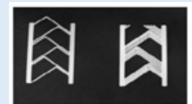
Herringbone spacer configurations as observed in literature. Shrivastava A, 2008
