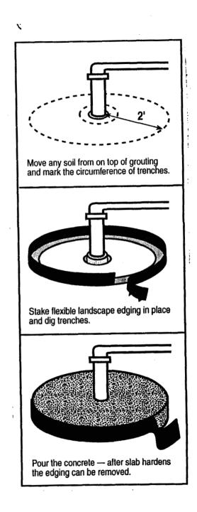
Figure 2. Side view of a typical well showing how flexible landscape edging can be used as a form for curbing.
