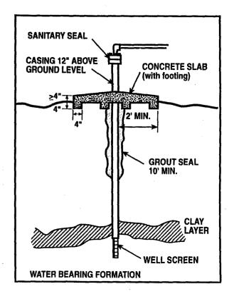
Figure 1. Cross sectional view of a typical well showing proper construction to prevent contamination
