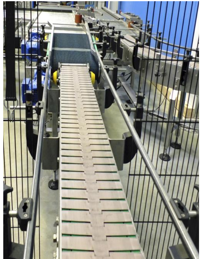
Kastentransport Crate conveyor
