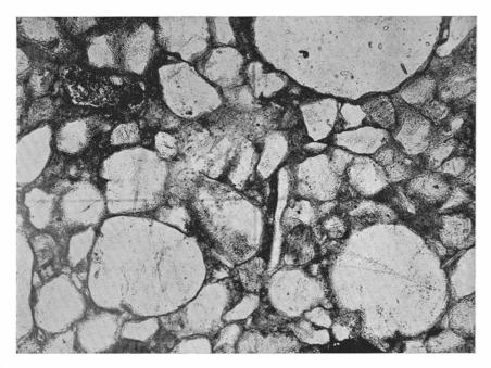
Fig. 66. Coarse-grained quartz sandstone. Lower Cambrian basal layer. Pessinenjokk, Luopahta, Lapland. 60 X. (Pr. 906. Pl. 382.)
