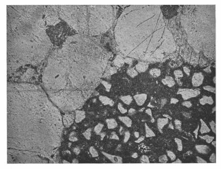
Fig. 12. Sandstone with phosphorite on secondary deposit. Phosphorite nodule, containing small angular quartz grains, embedded in a coarse-grained calcareous sandstone with well rounded quartz grains. Lower Cambrian. Hardeberga. (Pr. 2683. Pl. 341.) — 60 ×.
