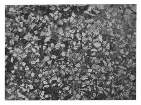
Fig. 65. Fine-grained sandstone with quartz cement. Lower Cambrian. Pessinenjokk Luopahta, Lapland. 60 X. (Pr. 904. Pl. 381.)
