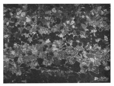
Fig. 92. Calcareous sandstone with pyritic laminae. Lower Ordovician (Dictyograptus shale). Storberg,  $\Theta$ stergötland. (Pr. 627. Pl. 288.) - 50 ×. Nic. +.
