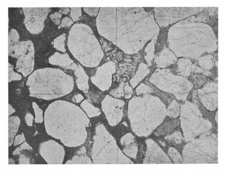
Fig. 1. Sandstone with rounded grains. Matrix silicified. Lower Cambrian. Luopahta, Lappland. (Pr. 2845. Pl. 383.)<sup>1</sup> - 60  $\times$ .
