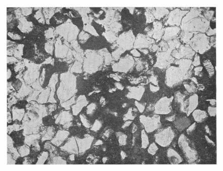
Fig. 11. Sandstone with phosphorite on primary deposit. The quartz grans are locally cemented by phosphorite. The lower right part of the fig. shows a small part of a phosphorite nodule containing an abundance of quartz grains of the same size and shape as in the surrounding rock. Lower Cambrian. Brantevik, 6. (Pr. 2796. Pl. 364.) - 60  $\times$ .
