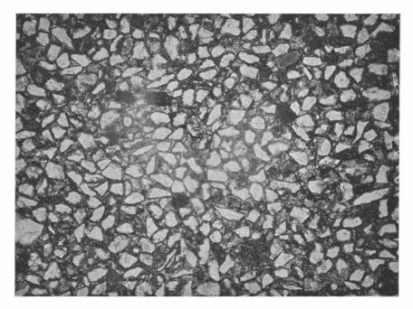
Fig. 9. Ferruginous sandstone. Small angular quartz grains cemented by siderite and limonite. Lias. The zone with Avicula inaeqvivalvis. Kulla Gunnarstorp, Scania. (Pr. 2549. Pl. 321.)  $-60 \times$ .
