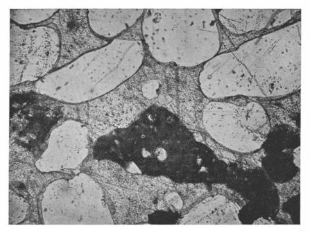
Fig. 5. Sandstone with matrix and cement of calcite, enclosing phosphorite and glauconite. Lower Cambrian. Brantevik, 9 b. (Pr. 2801. Pl. 363.)  $-60 \times$ .
