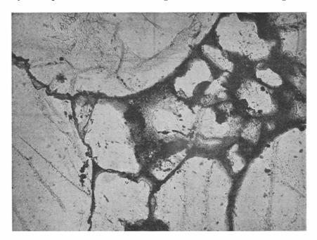
Fig. 3. Sandstone with a matrix of small angular rock fragments between the larger, rounded grains. Cement: calcium phosphate. Lower Cambrian. Simrishamn. (Pr. 2770. Pl. 370.) - 60 ×.
