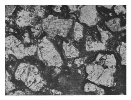
Fig. 104. Argillaceous and calcareous sandstone (arkose) with angular grains. Keuper. Hoby, Scania. (Pr. 665. Pl. 302.) - 60 ×.
