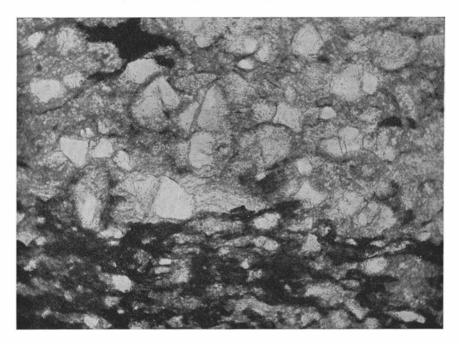
Fig. 71. »Hede limestone». Black argillaceous and gray arenaceous bands. Hede, Härjedalen. (Pr. 762. Pl. 385.)  $-60 \times$ .
