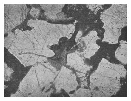
Fig. 2. Sandstone with angular grains. Matrix argillaceous. Keuper. Margreteberg, Höganäs, Scania. (Pr. 2505. Pl. 325.)  $-60 \times$ .
