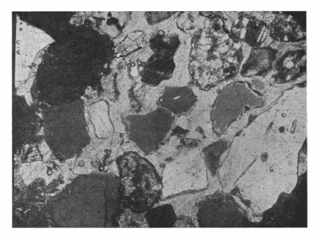
Fig. 107. Calcareous sandstone, red, with coarse-crystalline calcite cement. Keuper. Nyhamn, Scania. (Pr. 668. Pl. 300.) –  $50 \times .$  Nic. +.
