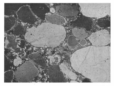
Fig. 4. Sandstone with a matrix of small quartz grains. Cement siliceous. The rock has macroscopically as well as microscopically a pronounced clastic structure. Lower Cambrian. Brantevik, loc. 4, Scania. (Pr. 2794. Pl. 359.) - 50 ×. Nic. +.
