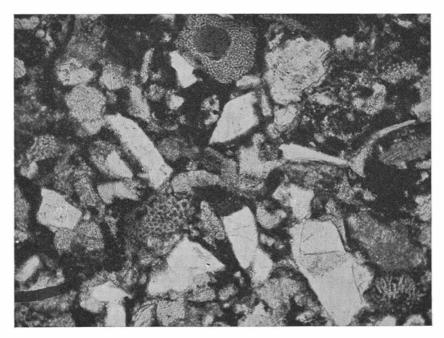
Fig. 86. Loftarstone. Fragments of fossils, shales, limestones and granite. Tandsbyn, Jämtland. (Pr. 691. Pl. 395.)  $-60 \times .$
