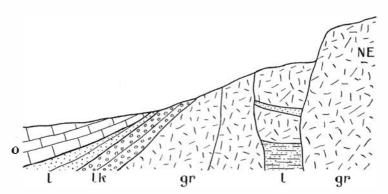
Fig. 90. Section 4. Granite horst, partly breccia-like, with faults and inclusions of fine-grained, stratified Loftarstone (washed-in material). The series of strata to the west in the section consists of Loftarstone resting on Loftarstone conglomerate and covered by limestone.
