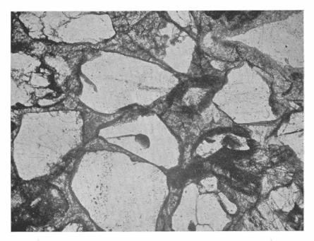
Fig. 10. Siderite sandstone. Angular quartz grains cemented by siderite. Lias. Fyledal, Scania. (Pr. 2859. Pl. 312.)  $-60 \times$ .
