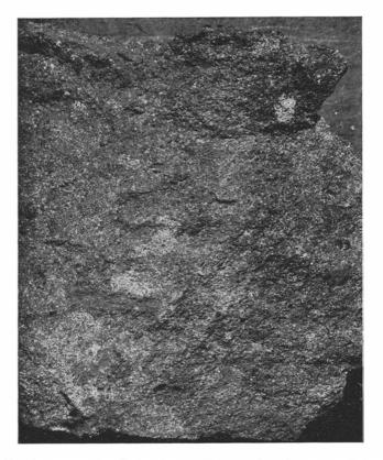
Fig. 106. Calcareous sandstone, red, with coarse-crystalline calcite cement. Some reflecting cleavage planes of calcite crystals are to be seen in the fig. Keuper. Nyhamn, Scania.  $-\frac{1}{1}$ .
