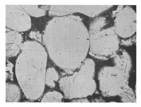
Fig. 7. Bituminous sandstone. Some of the quartz grains show secondary outgrowth. (See also fig. 53, 59 a. o.) Lower Cambrian. Karakås, Scania. (Pr. 2575. Pl. 373.) 60 ×.
