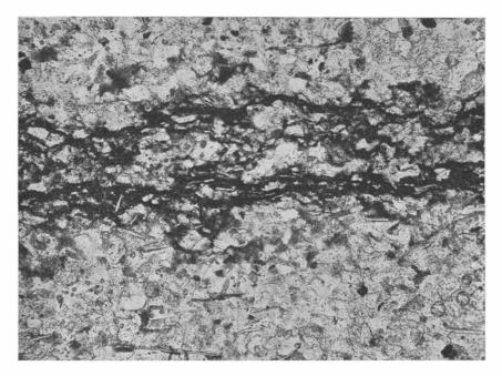
Fig. 56. Dark laminated sandstone with glauconite, pyrite and muscovite. Lower Cambrian. Brantevik, 6 b. 60 ×. (Pr. 2793. Pl. 358.)
