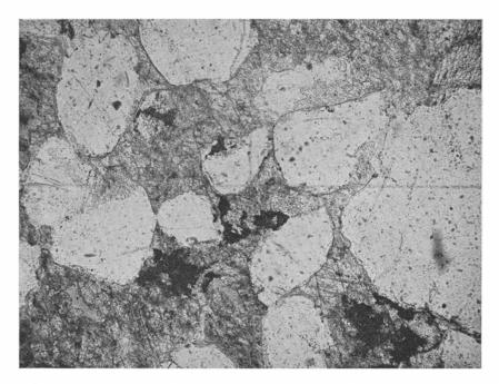
Fig. 8. Calcareous sandstone. Quartz grains cemented by fairly coarse crystalline calcite. Lower Cambrian. Karakås. (Pr. 2576. Pl. 374.)  $60 \times$ .
