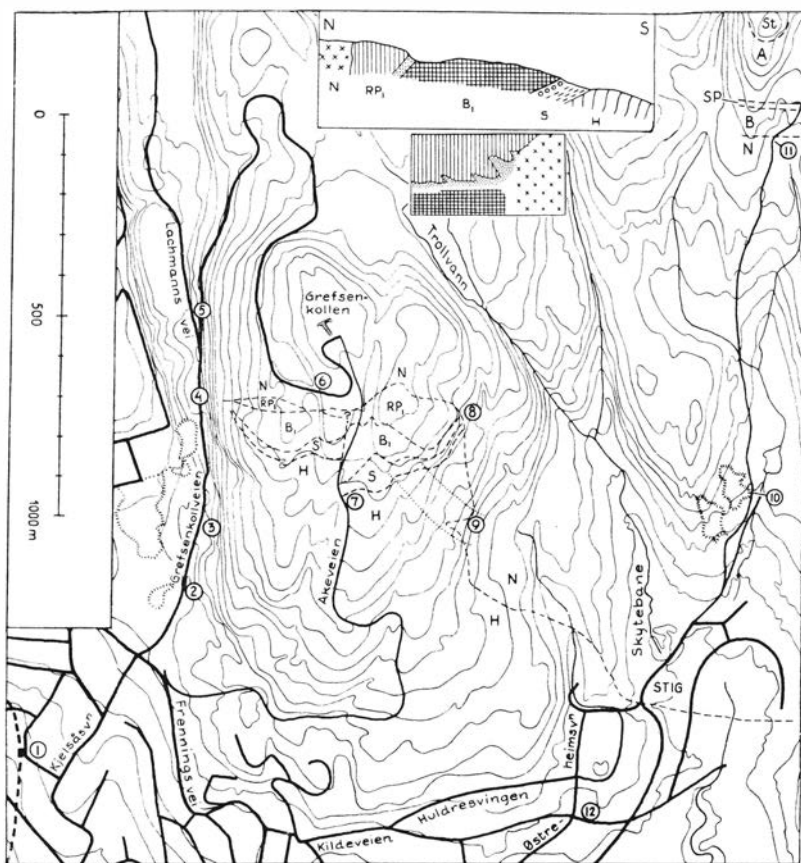
Fig. 38. Map to excursion 14. Upper section SW of (6). Lower section SW of (8), direction SW-NE, length about 20 m. H — hornfelsed Ordovician strata, S — basal Permian sediments, B 1 — basalt, RP 1 — rhomb porphyry, N — nordmarkite, B — basalt of Alnsjø area, SP — syenite porphyry, A — argillite and greywacke, St — summit of Storhaug (with conglomerate).
