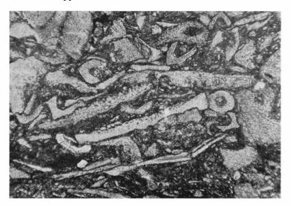
1. Thin section of the Dalby calcarenite. 34.2 % of fossil fragments longer than 0.1 mm in the thin section. Böda Hamn boring, between the levels of 1.97–2.00 m.  $\times$  40.
