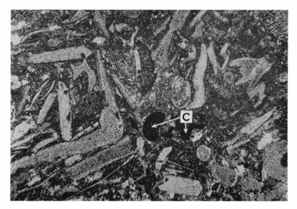
1. Thin section of the Folkeslunda calcarenite. Böda Hamn boring, between the levels of 13.47– 13.50 m. 27.8 % of fossil fragments longer than 0.1 mm in the thin section. C, chamosite filling a small gastropod shell. ×40.
