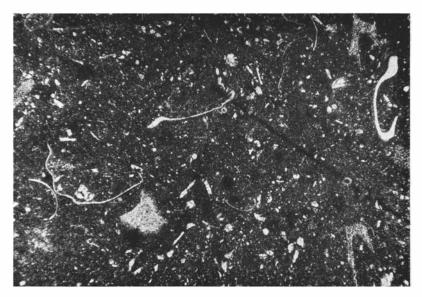
2. Thin section of calcilutite of the Furudal Formation. 5.9 % of fossil fragments longer than 0.1 mm in the thin section. Gammalsby boring, between the levels of 0.24–0.27 m. ×40.
