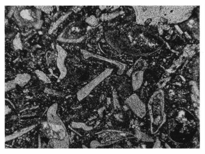
2. Thin section of the Persnäs calcarenite. 26.4% of fossil fragments longer than 0.1 mm in the thin section. Böda Hamn boring, between the levels of 10.00-10.03 m. The black colour within a gastropod shell in the lower right corner as well as the other black spots are caused by chamosite filling the cavities of shell fragments.  $\times 40$ .
