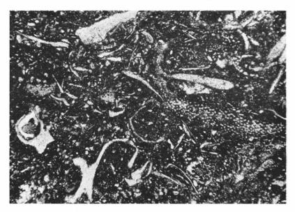
1. Thin section of the Källa calcarenitic calcilutite. 12.9 % of fossil fragments longer than 0.1 mm in the thin section. Böda Hamn boring, between the levels of 11.97–12.00 m. ×40.
