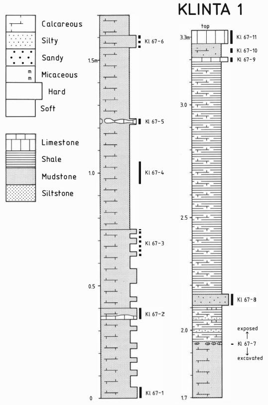
Fig. 7. Legend for Figs. 6-14 and lithostratigraphy and sample levels at Klinta 1. For details, see the text.
