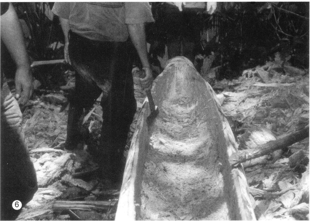
5. The softer inner material of the trunk is easily removed with a hatchet or machete. Photo by Jane MacKnight. 6. A view toward the bow of the nearly-completed canoe. Photo by Jane MacKnight.
