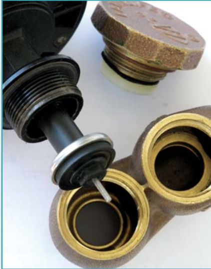
2. A disassembled brass irrigation valve showing the locations where small particles of sand and other debris can lodge and cause water leaks.
