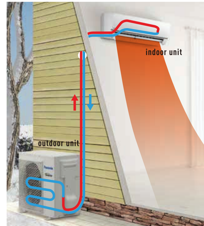
At heating operation Simply said, heat is transferred from outdoors to indoors using a compressor and high pressure, high temperature refrigerant. Cool air is drawn into the indoor unit and Warm air is released into the room. The refrigerant cycle continually repeats.
