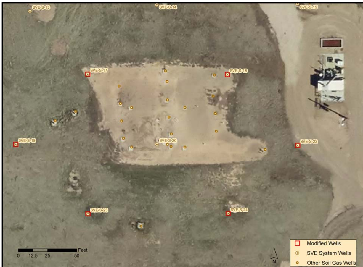
Figure 1-4. Burning Ground SVE System Wells and Modifications
