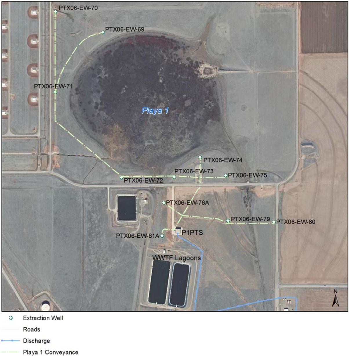
Figure 1-6. P1PTS Wells and Conveyance Lines
