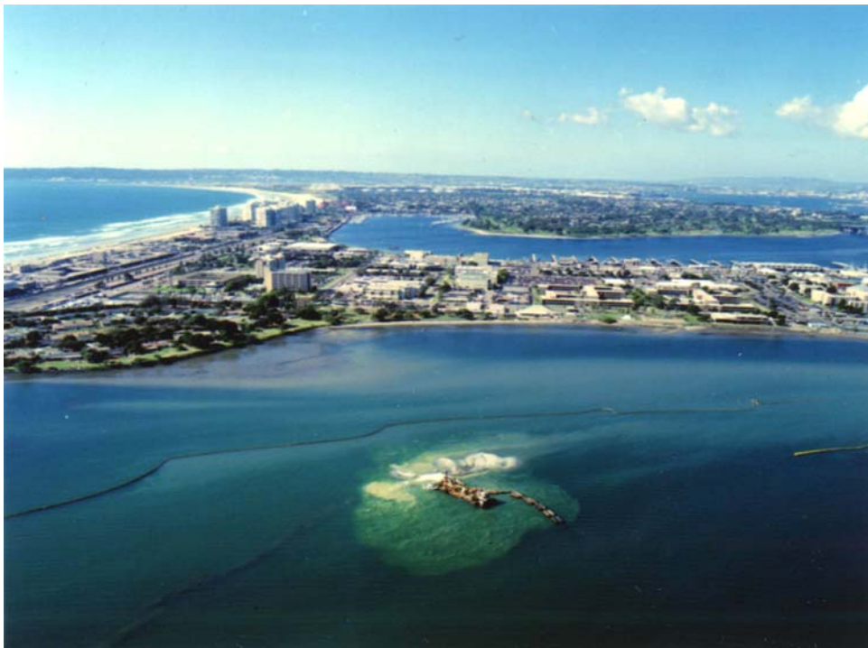
Photo 2-1. March 2001 oblique aerial of creation of Homeport Island as part of Navy nuclear carrier homeporting project. The photo shows three types of turbidity managers separate: ambient turbidity throughout the water profile as evident adjacent to the mudflat in the photo's center-left; water surface turbidity (lighter color in water nearest island construction); and subsurface turbidity plumes, shown closest to the photo foreground.
