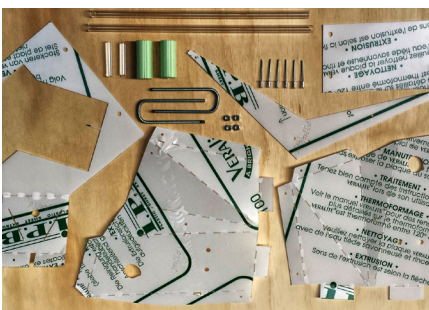
9 aPET Mold Components (Kristensen 2014)
