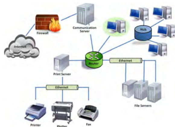
Figure 7.3: Typical wired local area network (Courtesy Department of Transportation)
