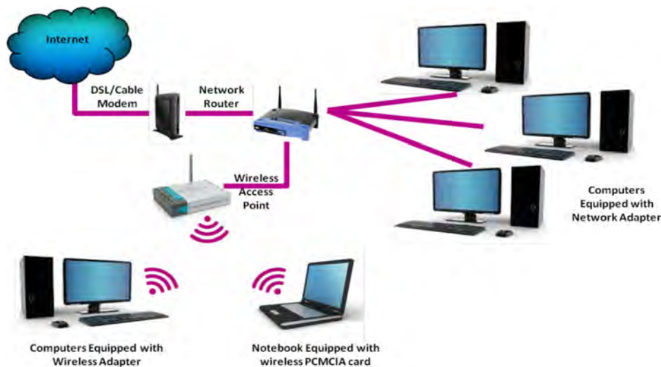
Figure 7.5: Wireless Local Area Network (WLAN) (Courtesy Home-Network-Help.com)
