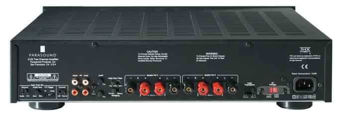
The Model 2125 is a Class AB amplifier designed for efficient, low heat operation. Its fully discrete circuitry is powered by a huge toroid transformer, and is capable of delivering 35 amps peak current per channel.
