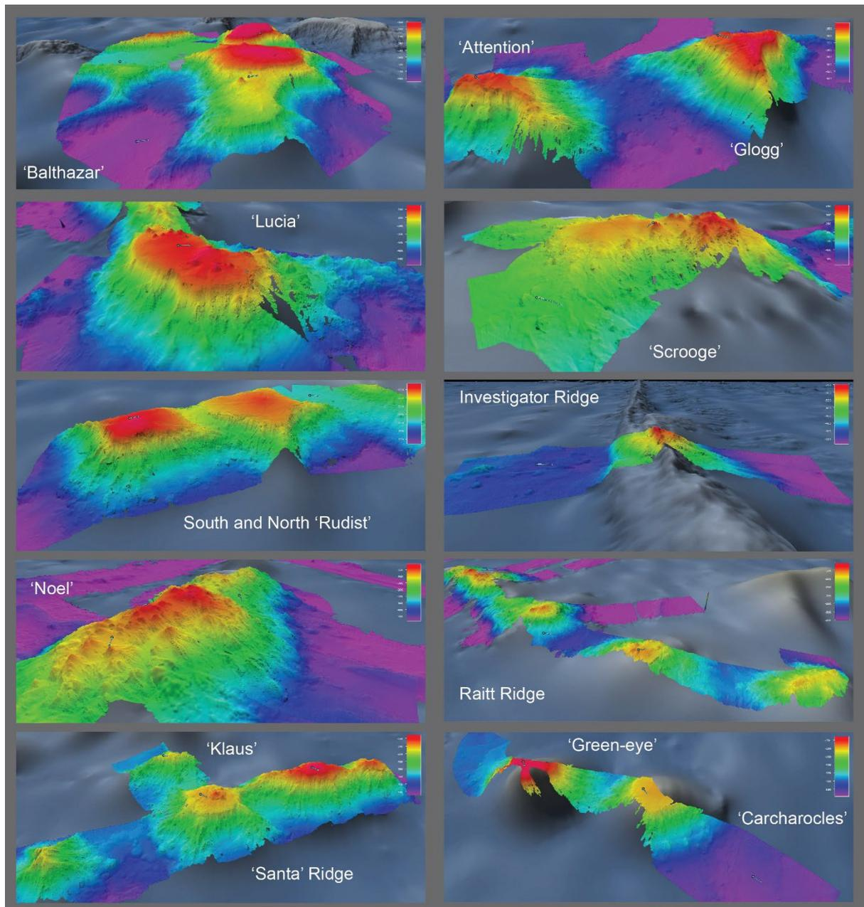
Figure 31B. 3d terrain representations of seamounts from the Christmas Island and Cocos (Keeling) Islands MPs derived from IN2022\_V08 expedition multibeam data (colour) overlain on GEBCO 2022 modelled bathymetry data (in grey). All orientations are from the south. 2.5x vertical exaggeration. Images: GSM/CSIRO
