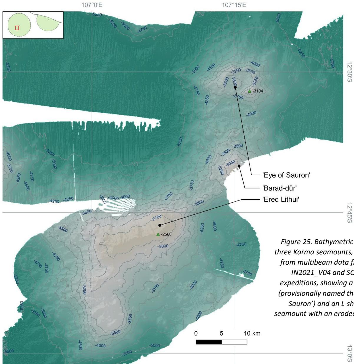
Figure 25. Bathymetric map of three Karma seamounts, compiled from multibeam data from the IN2021\_V04 and SO199 expeditions, showing a caldera (provisionally named the 'Eye of Sauron') and an L-shaped seamount with an eroded summit.
