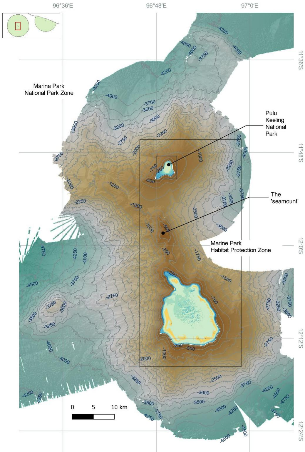
Figure 10. Bathymetric map of the Cocos (Keeling) seamount compiled from multibeam data from the IN2022\_V08 and SO199 expeditions. The topography of the two summits that rise above sea-level, the multi-island South Keeling atoll and North Keeling Island, are compiled from AHO LIDAR (LADS) data.
