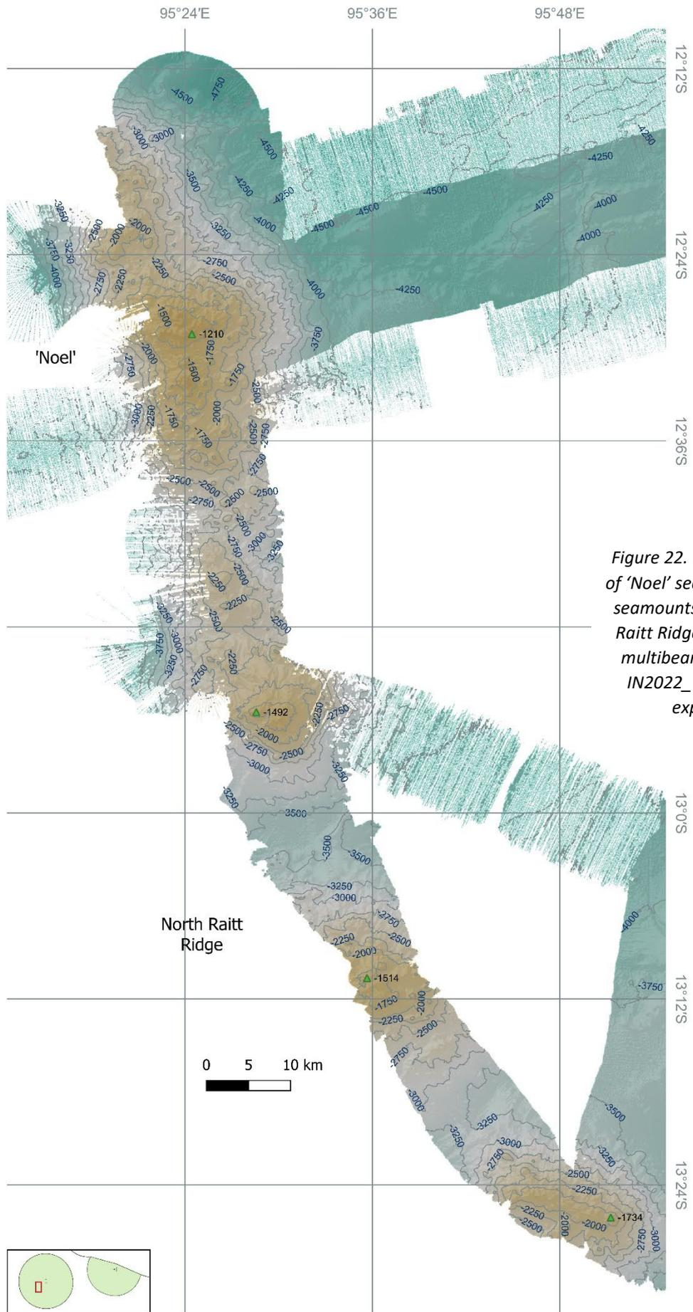
Figure 22. Bathymetric map of 'Noel' seamount and other seamounts on the northern Raitt Ridge, compiled from multibeam data from the IN2022\_V08 and SO199 expeditions.
