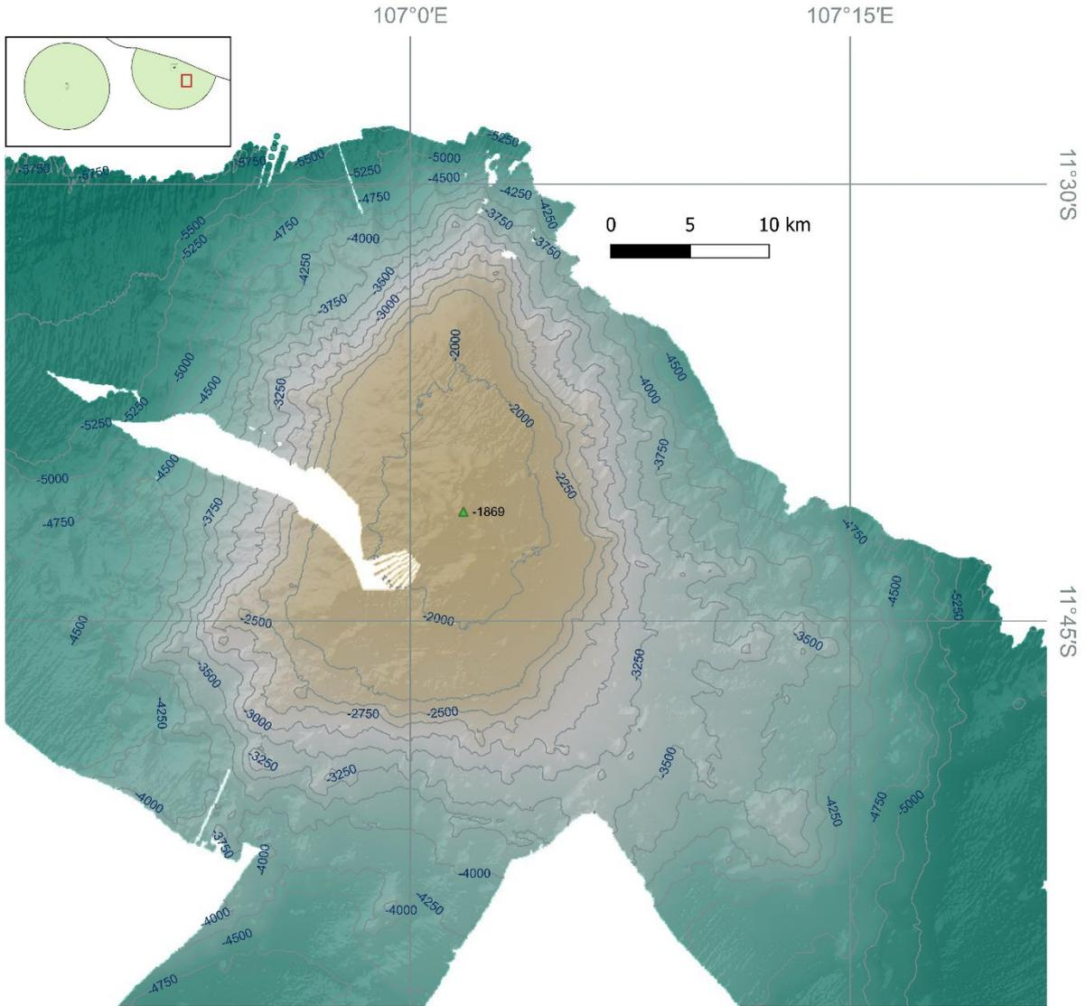
Figure 15. Bathymetric map of the 'Max' seamount, compiled from multibeam data from the IN2021\_V04 and SO199 expeditions, showing a large guyot-like seamount that summits above 2000 m depth with evidence of sediment erosion on the southern boundary.
