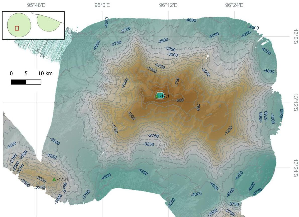
Figure 12. Bathymetric map of Muirfield seamount compiled from multibeam data from the IN2022\_V08 expedition and LIDAR data of the summit area. The summit (17.1 m) appears to be a drowned atoll sitting atop a limestone plug.
