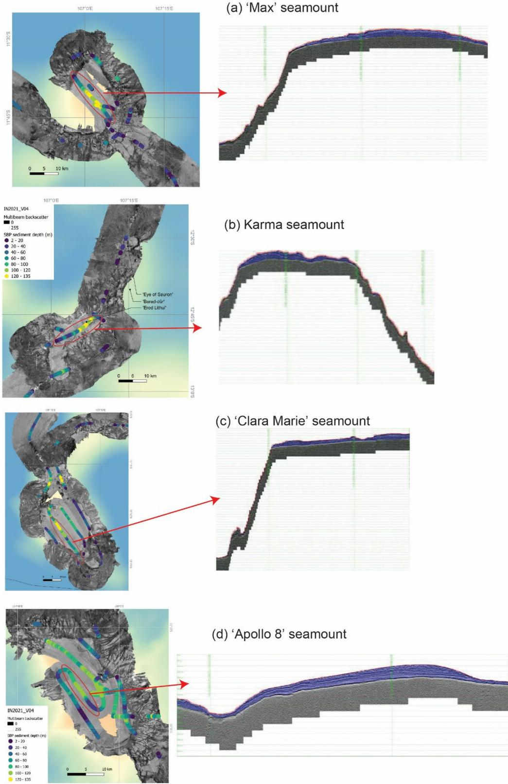
Figure 32. Sub-bottom profiles across selected seamounts in the Christmas Island Marine Park. The maps on the left show grey-scale multibeam backscatter data (black = relative hard, white = relative soft substrata) superimposed with coloured dots indicating the approximate depth of sediment. The sub-bottom profile of the transect within the red ellipses is shown on the right, with blue indicating depth of detectable sediment. Profile images GSM/CSIRO, maps MV.
