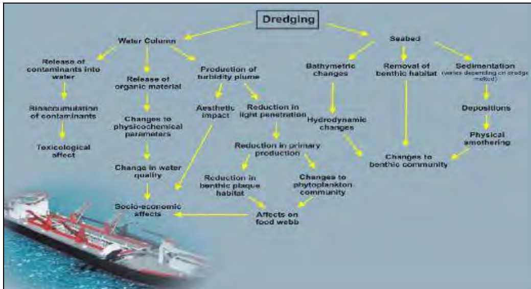
Figure 7.2 Conceptual diagram illustrating the impacts of dredging (Source: GHD 2005, after Elliot and Hemingway 2002)
