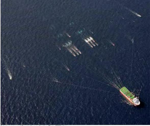
Seismic survey vessel for petroleum exploration. Photo: CGGVeritas.
