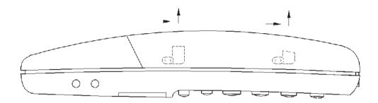
To open the battery compartment, press the cover with your thumb and slide towards the headset connection, then lift this upwards. To refit the cover follow this instruction in the reverse order.
