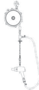
ATB-1 fitted with horizontal tool hanger
