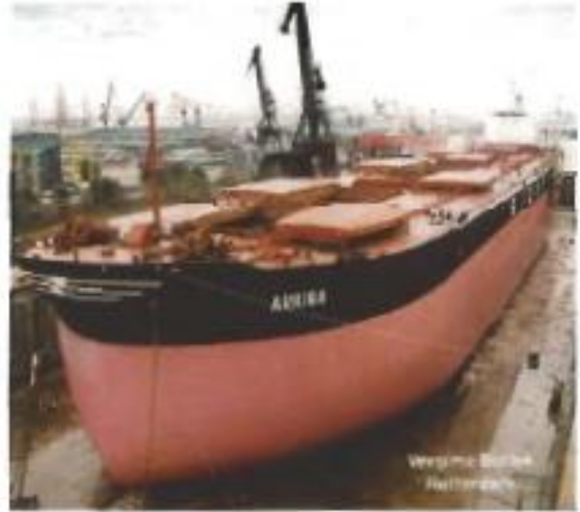
A ship with a large block coefficient but a large midship section coefficient
