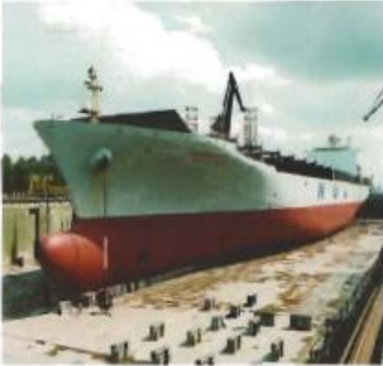
A ship with a small block coefficient but a large midship section coefficient
