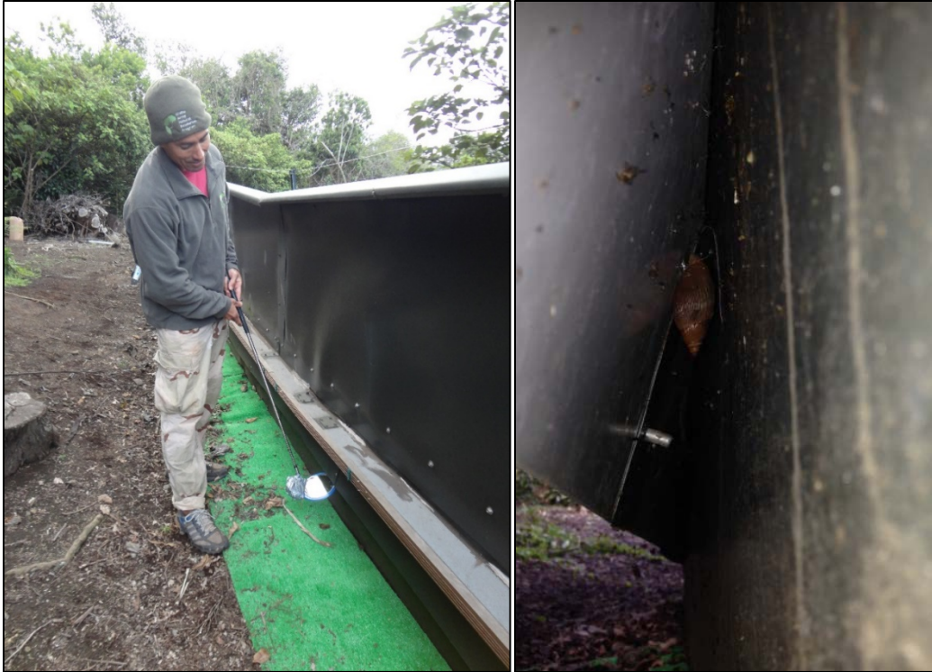
Figure 7. Monitoring of the angle barrier at Hapapa snail enclosure. The angle barrier at Palikea North enclosure is similarly monitored with the use of a mirror to view E. rosea trapped within it.
