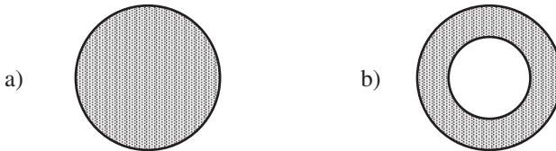
Figure 6.37. Current density of a cylindrical conductor far away from other conductor: a) low frequency; b) high frequency
