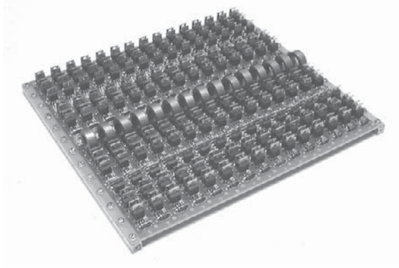
Figure 3.47. Board of MOS ON OFF CC, 5,000 V, 500 A
