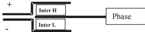
Figure 3.28. Use of busbar topology to reduce interconnection inductance (links high side switch H, low side switch L and DC bus capacitor)
