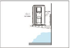
Fig 5.3.4. Outdoor Unit on Brackets above Snow Line
