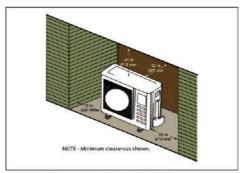
Fig 5.3.1. Unit installed in Alcove
