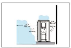
Fig 5.3.2. Outdoor Unit Air Flow Obstructed by Snow
