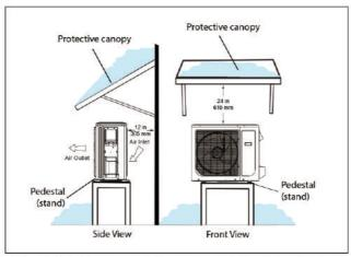
Fig 5.2.1. Outdoor Unit on Pedestal and Protective Canopy
