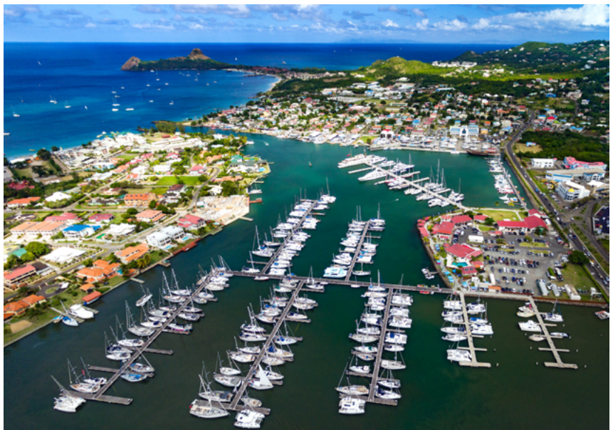
Saint Lucia, Rodney Bay Marina. Formerly a mangrove ecosystem, the mangroves were cleared and the area dredged. Dredged materials were used to construct a causeway to Pigeon Island (background). Credit: Kirk Elliot, Saint Lucia Photo Tours.
