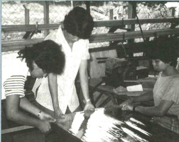
Polyethylene glazing is put on the solar dryer collector.
