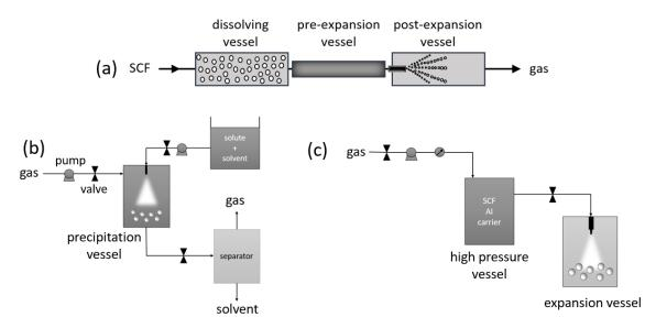
**Figure 2.** Shematic representation of SCF micronization processes: (a) RESS, (b) SAS, and (c) PGSS<sup>TM</sup>. Adapted from [32–34].
