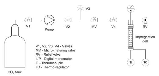
the drug into the polymer matrix [121]. Afterwards, depressurization allows the  $CO_2$  to change into a gaseous state upon venting, and the impregnated polymer can be recovered.
