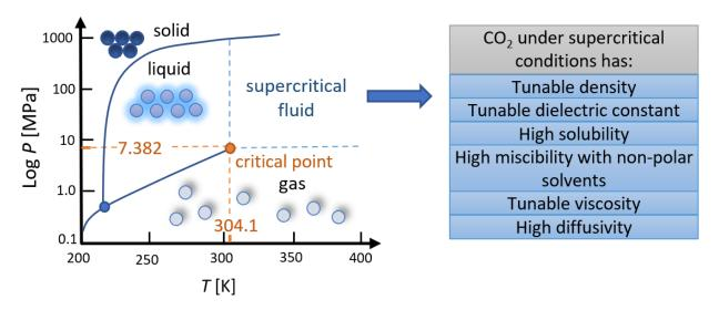
**Figure 1.** Phase diagram of CO<sub>2</sub> and its advantageous characteristics at supercritical conditions. Adapted from [22].
