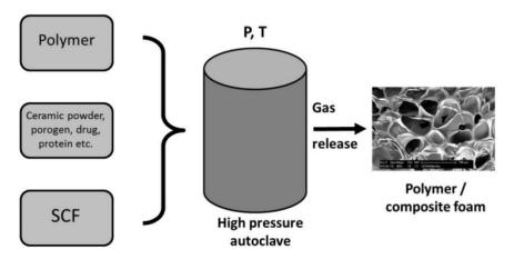
**Figure 5.** An illustration of the SC foaming leading to stabilized polymer/composite foams [105]. Reprinted from the Energy, 77, Knez et al., industrial applications of supercritical fluids: a review, 235–243, Copyright (2014), with permission from Elsevier.
