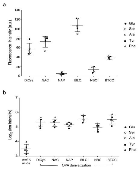
**Figure 2.** Fluorescence intensities (**a**) and ion intensities (**b**) of the OPA/thiol-derivatized L-amino acids (Glu, Ser, Ala, Tyr, and Phe) at equal concentrations. The center bar represents the mean, and the whiskers represent  $\pm 2$  standard deviations.
