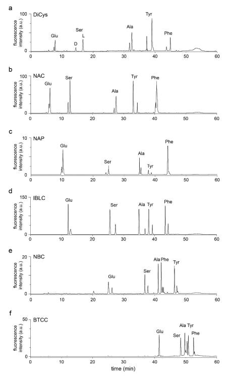
**Figure 3.** RP-HPLC analysis of amino acid enantiomers derivatized with OPA/thiol. The adducts of DiCys (a), NAC (b), NAP (c), IBLC (d), NBC (e), and BTCC (f) are detected by 340 nm excitation/450 nm emission. The ratio between L:D amino acids is 3:1.
