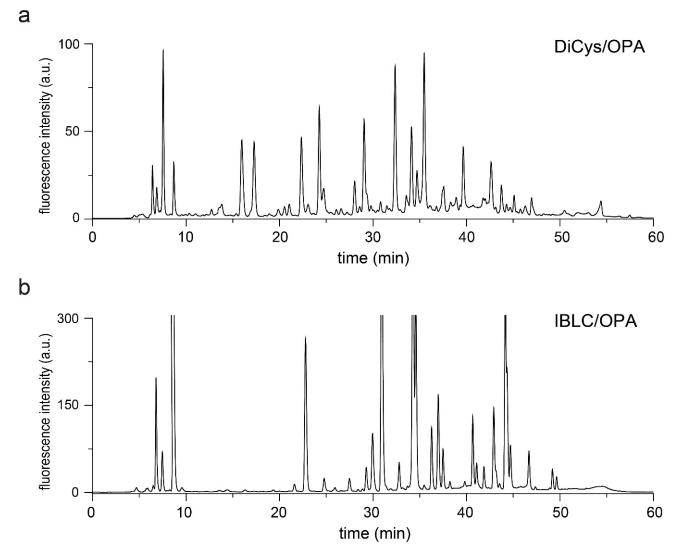
**Figure 4.** RP-HPLC analysis of free amines in rice water derivatized by DiCys/OPA (**a**) and IBLC/OPA (**b**), detected by 340 nm excitation/450 nm emission.
