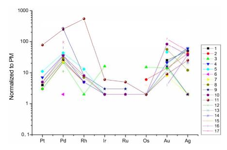
**Figure 3.** Primitive mantle-normalized [21] spidergram of the platinum-group elements (PGE), Ag and Au content in the rocks of the Guli Intrusion (for the description of the numbers, see Table 3).
