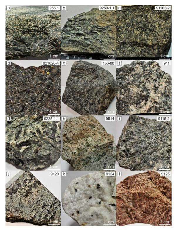
**Figure 2.** Photographs of the main rock varieties: (**a**) meimechite; (**b**) dunite with chromite schlier; (**c**) ore wehrlite; (**d**) ore pyroxenite; (**e**) kugdite; (**f**) ijolite-melteigite; (**g**) coarse-grained shonkinite; (**h**) alkaline microsyenite; (**i**) foyaite; (**j**) magnetite-apatite-diopside rock; (**k**) calcite carbonatite; (**l**) dolomite carbonatite.
