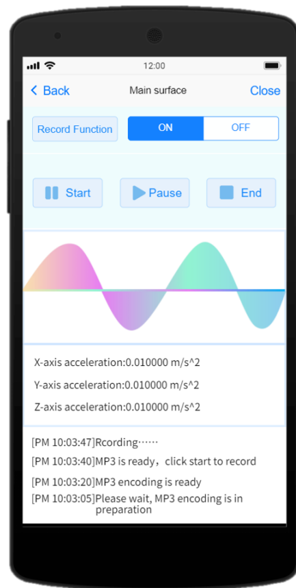
Figure 3. Main interface of the data acquisition module.
