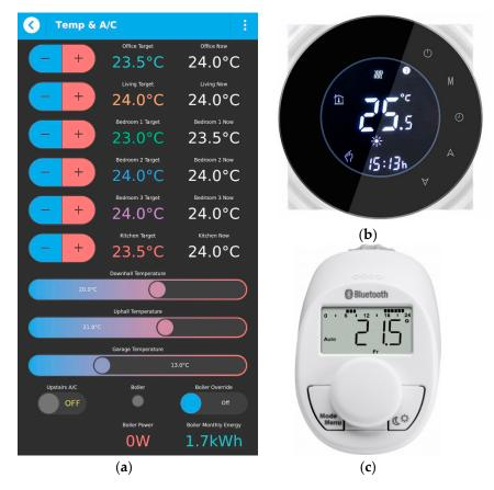
Figure 8. Controlling indoor temperatures with qToggle app (a) together with smart termostats (b,c).
