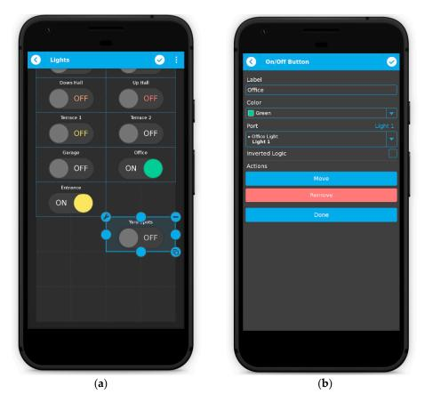
Figure 5. Working with widgets: dashboard layout (a), widget properties (b).
