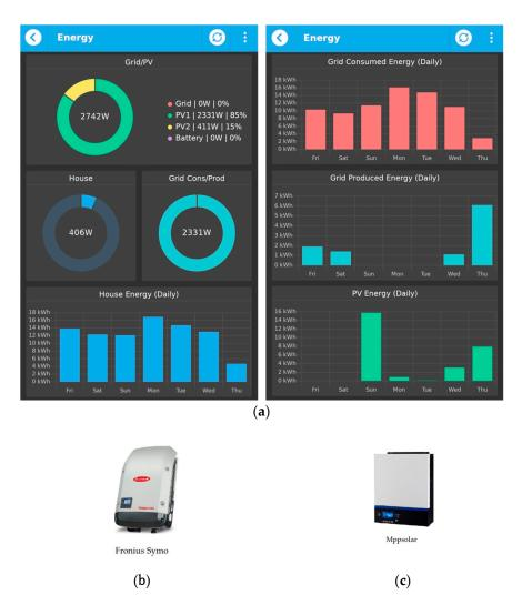
**Figure 10.** Monitoring the energy with qToggle (**a**) and the two invertors: Fronius Symo (**b**) and Mppsolar (**c**).
