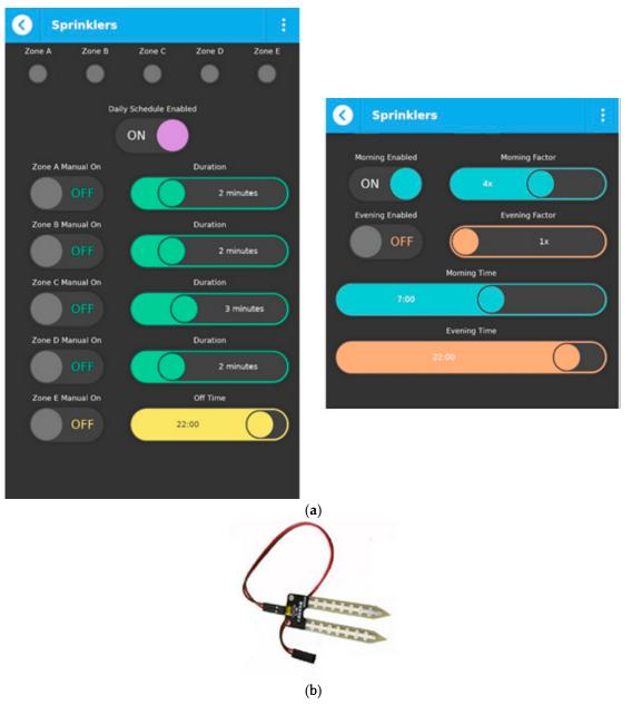
Figure 13. Controlling the irrigation system with qToggle (a) and the YL 69 sensor (b).
