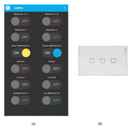
qToggle is compatible with Amazon Alexa as well. The devices used for controlling the lights are Sonoff Touch with one, two, or three channels.
