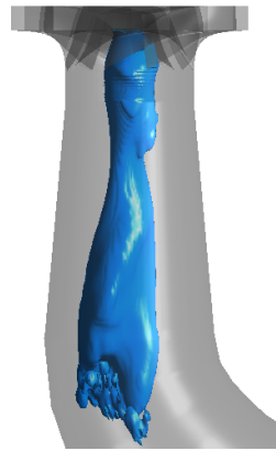
Figure 11. The cavitation area in the draft tube.
