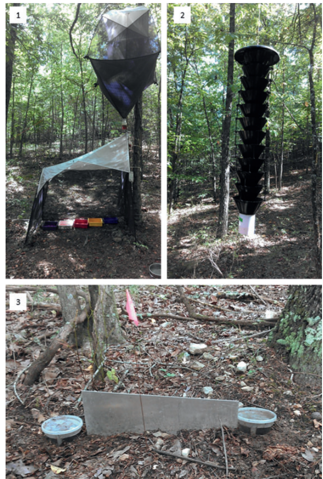
Figs. 1–3. Examples of traps used. (1) Malaise trap with pan traps underneath acting as intercept traps and a S.L.A.M. canopy trap. (2) Black Lindgren funnel trap. (3) Pitfall set. The canopy trap and Lindgren funnel trap were lowered from the canopy for the photographs.
