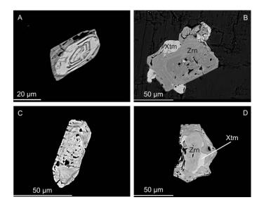
**Figure 7.** High-contrast BSE images of zircon (Zrn) and xenotime (Xtm) from granites of the Krudum granite body. (**A**) Oscillatory zoning of zircon from the medium-F biotite granite, (**B**) Intergrowth of xenotime with zircon from the high-F, high- $P_2O_5$  Li-mica granite, (**C**) Oscillatory zoning of altered zircon in the high-F, high- $P_2O_5$  Li mica granite, (**D**) Inherited zircon grains overgrown by younger zircon and xenotime from the high-F, high- $P_2O_5$  Li-mica granite.
