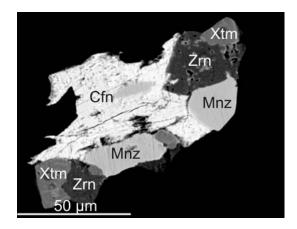
**Figure 6.** High-contrast back-scattered electron (BSE) image of complex intergrowths of coffinite (Cfn), zircon (Zrn), monazite (Mnz), and xenotime (Xtm) from high-F, high-P<sub>2</sub>O<sub>5</sub> Li-mica granite, Hub stock.
