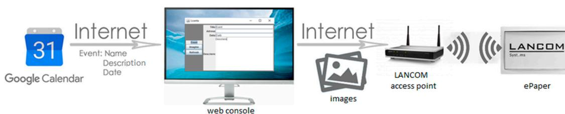
Figure 1. Typical SICIAD ePaper displaying scenario.
