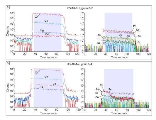
**Figure 15.** Representative single-spot LA-ICPMS spectra (blue shading) for selected elements in homogenous low-Hg sphalerites without mineral inclusions (**a**) and with Pb-Sb-Cu-(Ag) sulfosalt micro-scale inclusion (**b**). For sphalerite compositions, see Tables 4 and 6.
