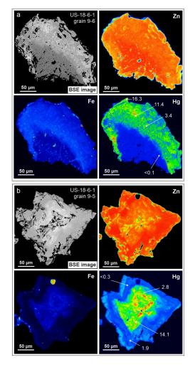
**Figure 13.** Back-scattered electron (BSE) images and element maps (Zn, Fe, Hg) of irregular (**a**) and zonal (**b**) distribution of Hg in South Sakhalin MV sphalerite. The numbers show Hg contents in wt% (WDS-EDS data). For representative compositions of the grains see Tables 4 and 6.
