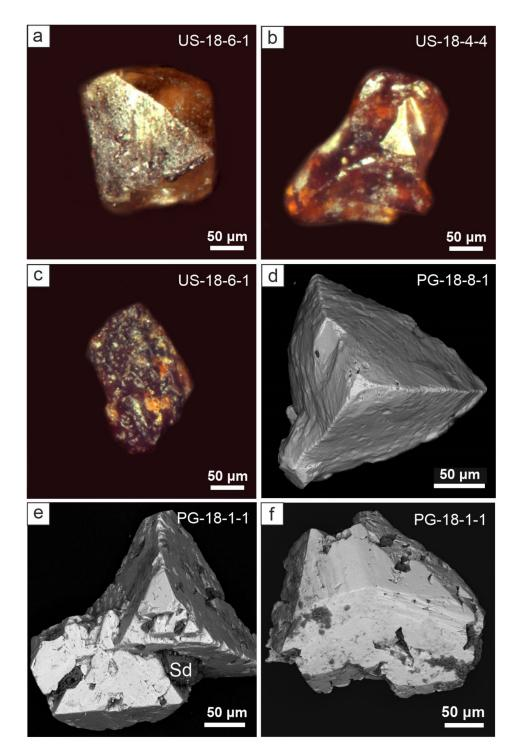
**Figure 9.** Appearance and morphology of low-Hg (<0.3 wt%) sphalerites from mud masses of South Sakhalin (**a**–**c**) and Pugachev (**d**–**f**) MVs. Optical images: (**a**) pseudo-octahedron, (**b**) intergrowth of tetrahedrons, (**c**) irregular fragment of heavily etched grain. BSE images: (**d**) tetrahedron with rounded and slightly etched tetrahedron surface, (**e**) intergrowths of sphalerite tetrahedrons with clay matter and siderite, (**f**) trigon-tritetrahedron. Sd = siderite.
