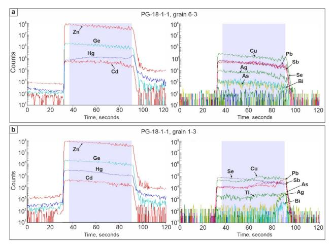
**Figure 16.** Representative single-spot LA-ICPMS spectra (blue shading) for selected elements in heterogeneous medium-Hg sphalerites without mineral inclusions (**a**) and with Pb-Sb-(Cu-Ag-Bi) sulfosalt and/or galena inclusions (**b**). For details of Hg distribution see Figures 11 and 13. For sphalerite compositions see Tables 4 and 6.
