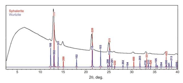
**Figure 17.** The powder diffraction pattern generated from the frames of a single crystal diffraction experiment of Mongolian high-Hg sphalerite in comparison with calculated powder diffraction patterns of sphalerite (red line) and wurtzite (blue line).
